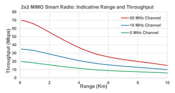
**Reference Configuration:** Cross-polarized H and V antennas for maximum diversity. Flyer antennas with E-tilt down and GCS antennas with E-tilt up. >15 dBm fade margin used in calculations to account for changing RF conditions.
